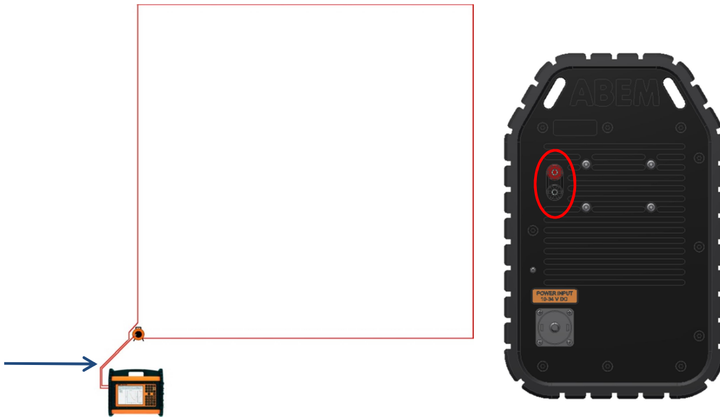
Figure 10. Transmitter loop is connected using the 3 meter lead-in cable. This permits the instrument to be placed 3 meters away from the transmitter loop and the electromagnetic field it generates.
