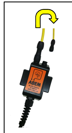
Figure 13. The RC-200 receiver cord is routed in a clockwise direction starting from the disconnectable plug.
