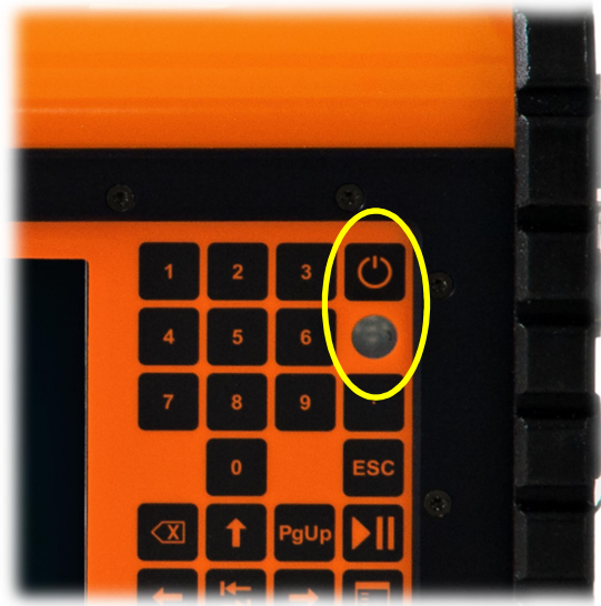
Figure 21. The location of the power on/off button and power indication lights on the ABEM WalkTEM
