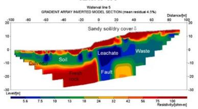
THE UPPER MODEL SECTION SHOWS THE RESISTIVITY RESULTS AND IT CAN CLEARLY BE SEEN THAT BY USING RESISTIVITY ALONE IT IS NOT POSSIBLE TO DETECT WHERE THE WASTE IS LOCATED AS THE WASTE LOCATED IN THE RIGHT PART OF THE SECTION HAS APPROXIMATELY THE SAME RESISTIVITY AS THE SOIL IN THE LEFT PART OF THE SECTION.
