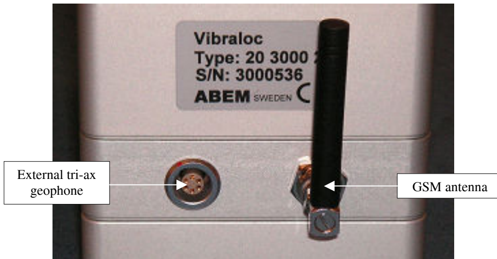
Figure 14. Connections for external tri-ax geophone and GSM antenna
