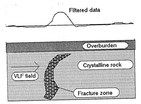
The upper figure shows the typical behaviour of an original VLF anomaly: a maximum occur to the left and a minimum to the right of the conductor. The above sketched anomaly can be imagined to be the real part, i.e. that part of the resulting field which are in phase with the primary field from the VLF transmitter. (The WADI instrument will also measure an imaginary component which are 90° out of phase with the primary field).
