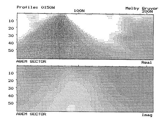
The lower two figures on the previous page shows a vertical cross section from the actual profile. This section is calculated by running the filtering process at successively increasing depth, and representing the calculated value (i.e. equivalent current density) by a grey shading. From this plot we conclude that the zone is quite shallow and slightly dipping towards South. It appears to be easy to set a drill hole based on this representation.
