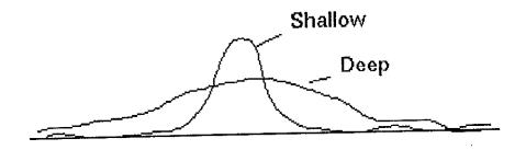
We observe that for a conductor at greater depth, the width of the anomaly will increase and the height will decrease. A small amplitude can, however, also be caused by a conductor which is not a very good conductor.
