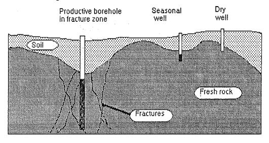
Highly productive water wells are obtained by drilling in rock that is broken along joints and small fractures. The WADI finds structures where useful quantities of underground water may be trapped in rock fractures and cavities, thus enabling drillers to select the most promising sites for their wells.
