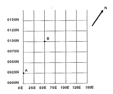
In the next example a visible strike direction is observed (in the vegetation or in the topography). The strike direction is approximately in the East-West direction, and you plan to make some WADI profiles perpendicular to the interesting area.
