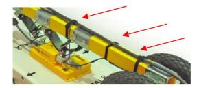
The MALÅ HF antennas (1.2, 1.6 and 2.3 GHz) are mounted on the black plastic HF holder which again is attached in-between the wheels of the MALÅ RoadCart.
