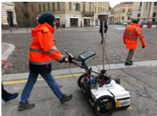
The measurement set-up with a hand towed solution. Note that the GPS could not be used in this urban area, crowded with high buildings.
