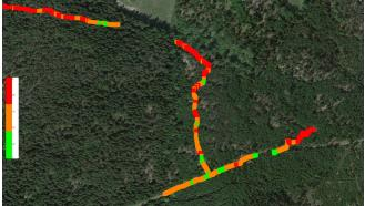
The results were visualized in Google Earth in an easy colourscale showing the locations of shallow to deeper bedrock levels clearly.
