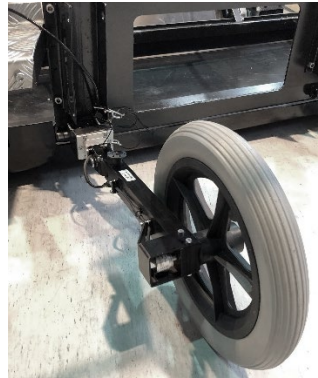
Vehicle mounted encoder and the 300mm measuring wheel.
