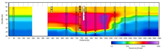
Based on the geophysical results, a preliminary interpretation of the limestone bedrock interface is produced:
