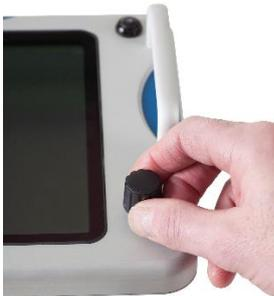
The GX Controller is operated with a dual function **Navigator** for selecting options and functions. Menu items are selected by rotating the Navigator clockwise or anti-clockwise. The selected item is then executed by pushing the button
