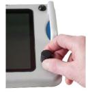
The GX Controller is operated with a dual function Navigator for selecting options and functions. Menu items are selected by rotating the Navigator clockwise or anti-clockwise. The selected item is then executed by pushing the button. For fast scroll, press, hold and rotate.
