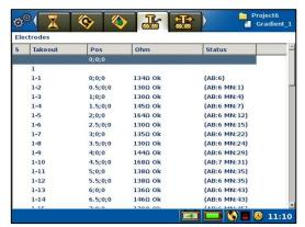
Note that this shows a spread with 0.5m electrode spacing
