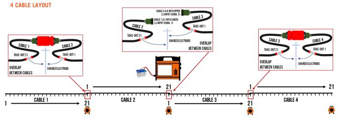
See pages 4 & 5 of this Quick Guide for details on how to use the 4x21 cable set to its full capacity
