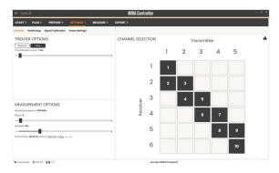
Make sure your MIRA system is connected to a high accuracy positioning system (RTK-GNSS or Total Station). Positioning settings are available in the *Positioning* tab.
