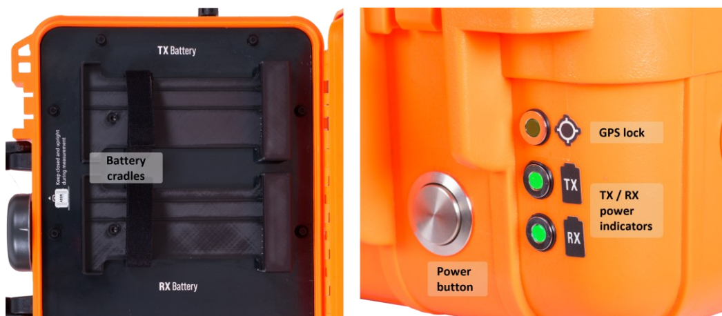
Figure 4. GroundTEM i-Series unit. Battery cradles and battery LED lights when batteries are inserted.
