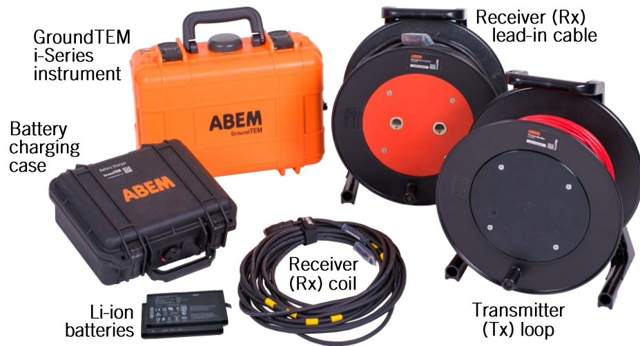
Figure 3. Main components of the GroundTEM system (note that GroundTEM i20 has three Li-ion batteries).
