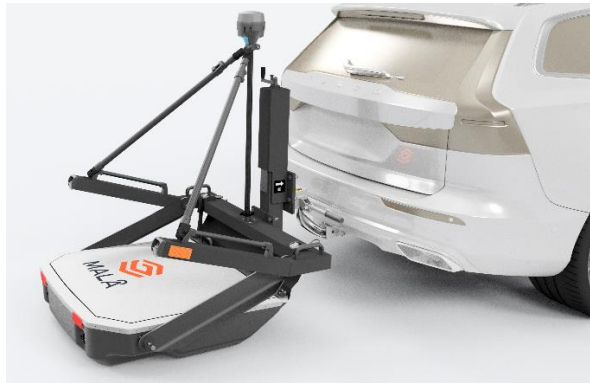
Car mount in measurement mode
